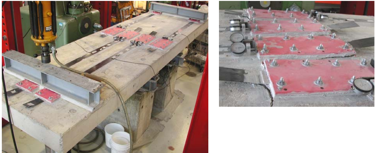
Fig. 10 Test slab for fatigue testing of the anchorages, anchorages after slab failure still intact.
